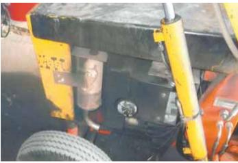
Home-built muffler was made by cutting 16 in. off a 4-in. dia. grain auger and welding a length of flighting inside. A curved exhaust outlet is bolted on at bottom.
