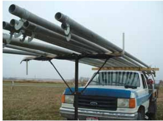
Home-built irrigation rack hauls 40-ft. long irrigation pipes on 1-ton pickup.
