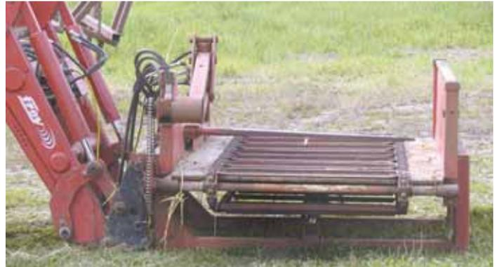
Edgar used unloading chain from a forage wagon to make unloader.
