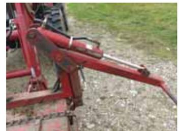
Unroller slides out to either side for unloading into pens. Bale spear reaches out to the left side of tractor to load bales onto platform.
