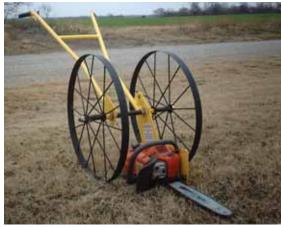
"Chainsaw Caddie" provides a way to hold and maneuver a chainsaw close to the ground, so you don't have to bend over, stoop or carry the chainsaw.
