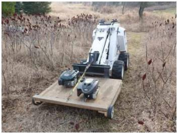
He removed the engines and blades from two 6 1/2 hp push-type, 21-in. mulching mowers, then mounted the engines on the wooden deck.
