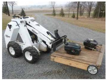
Dave Kulzer built this 40-in. wide, skid loader-mounted brush cutter out of wood. Loader forks slide through a pair of slots cut into back of deck.
