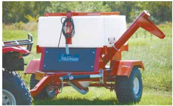
A handheld remote controls wagon's twin-speed auger. Works great for augering into bunks, dumping on the ground or filling buckets.
