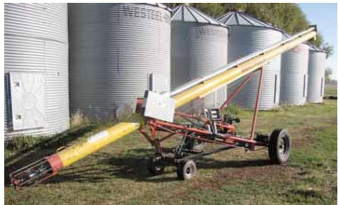
Brent Litke made this auger mover out of an old riding mower. "I stand next to the auger and use toggle switches inside a control box to control all operations," he says.
