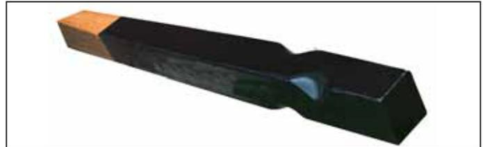
Smart Post plastic wrap is designed to protect wood or steel posts from moisture. To install you apply an adhesive coat to post, and then slide a plastic bag over it.
