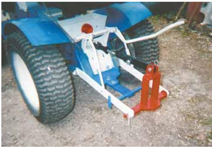
To make this 3-pt. mounted drawbar, Seltzer welded a length of rod to a flat piece of steel that hooks onto the tractor's original 3-pt. hitch. The rod supports the 3-pt.'s lower lift arms so they can't drop down too far.
