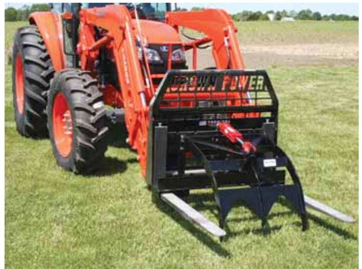
Add-A-Grapple comes with its own hydraulic cylinder and attaches to standard pallet forks with a screw-on lockdown clamp and a locking pin.
