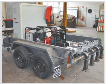
Microwave weed zapper uses four microwave generators powered by portable genera-tors. The microwave treatment "explodes" cells in weeds, to kill them.
