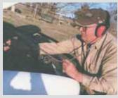
own inexpensive tester using a pair of ear muffs I bought at Harbor Freight. On one side I drilled a 3/8-in. dia. hole and inserted a length of 1/4-in. dia. tubing. I taped a length of small dia. pipe to the other end of the tubing. Now I can probe around the engine and hear the vacuum leak, which makes a hissing sound in the ear muffs.
