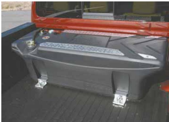
**Poly auxiliary fuel tank can be fitted with a hose and nozzle to fill other vehicles.**
