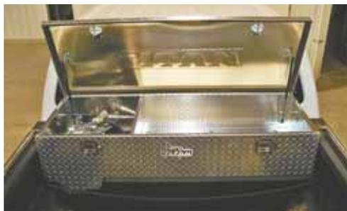
**Optional toolbox can be fitted to top of fuel tank.**
