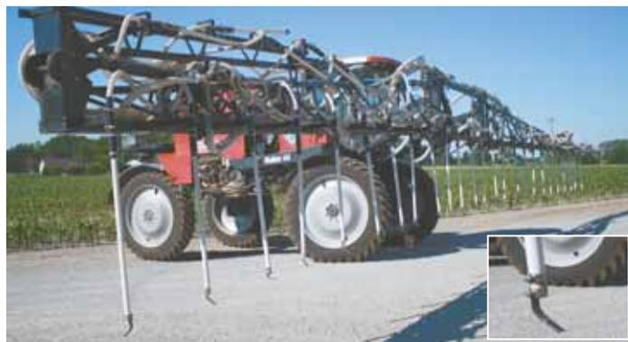
**Matt VanTilburg converted this Walker self-propelled sprayer to seed cover crops in corn and beans. Seed is blown down close to the ground through 3-ft. pvc drop tubes.**
