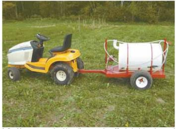
LeRoy Momper put together this small sprayer using a 55-gal. plastic barrel mounted on a trailer. Boomless spray nozzle at the rear sprays a 16-ft. wide pattern.
