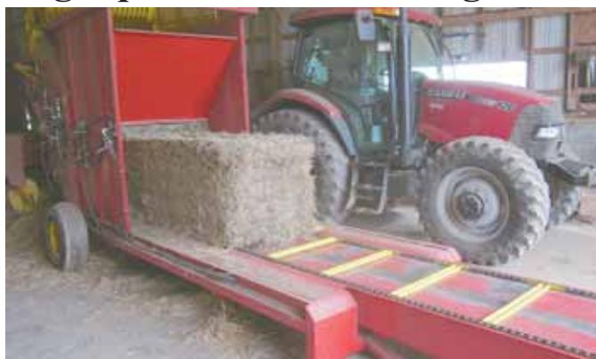
**Hydraulic-operated apron chain feeds bales into machine, which tears them apart and sends loose hay out the back. There it's fed into a baler making small square bales.**
