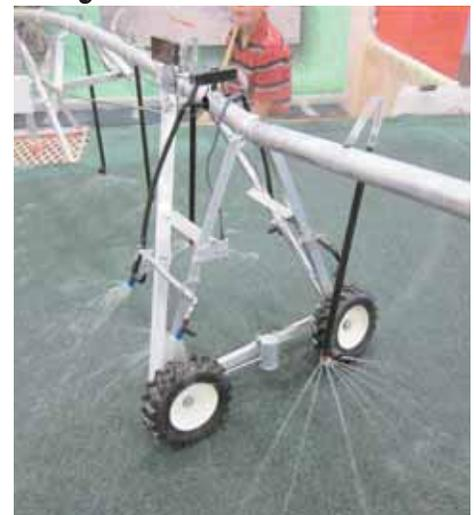
**Auto Dry Track System stops ruts before they start by using half nozzles to spray water to the sides and back of tires.**
