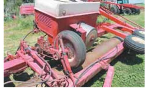
“I mounted an IH Cyclone box on top of each roller, with their drive wheels running on the rollers,” says inventor Brian Hoogestraat.
