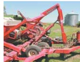
A 3-section frame built out of 7 by 7-in. sq. tubing supports both the rollers and planter units.
