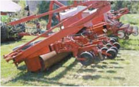
“Pave and plant” rig rolls fields and plants in a single pass. Planter units mount behind 24-in. dia. rollers, creating a tabletop-smooth surface for planting.
