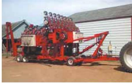
Folding the wings into transport position causes planter units to raise into a vertical position.
