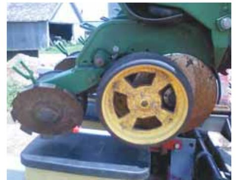
Hoogestraat cut holes into his planter’s gauge wheels so they don’t plug up with mud. He also converted disc openers into notched closing wheels for better traction in mud.
