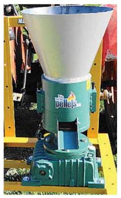
Pto-powered pelletizer has a heavier-duty gearbox that'll stand up to increased pellet-making torque, says the company.
