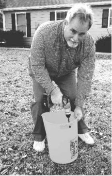
Collector tube extends up from bottom of bucket. To collect soil sample, the operator runs a cordless drill-powered auger through tube and into the ground.
