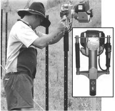
Hammer action on this handheld post driver is provided by a Honda GX35 gas engine, eliminating the hoses needed for hydraulic or air-powered drivers.
