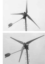
Win-Pressor turbines are designed to produce compressed air instead of electricity. Photo at upper left shows unit in gear. Photo at lower left shows unit furled and out of gear.
