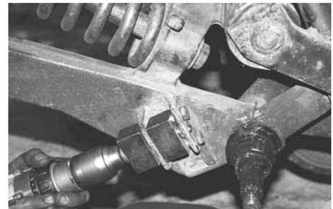
Repair involves drilling out the hole on seed boot mounting lug, then installing a hardened full length bushing.
