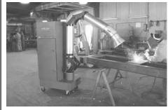
Air cleaner rides on four caster wheels. Suction arm on front draws dirty air into the unit before it has a chance to get out into shop.
