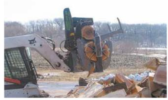
System lets operator pick up whole logs, saw them to firewood lengths and split the blocks, all without leaving the skid steer seat.
