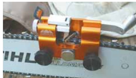
Timberline's crank-type chainsaw sharpener comes with a carbide cutter that rides the bar. The operator pulls the chain through to sharpen each tooth.
