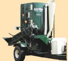
Art's Way Portable Grinder/Mixers are available with either hammermill or rollermill action to grind feed into a consistent and uniform ration. Choose from the 105 bushel or the large 165 bushel tank to grind and mix up to 4 ton of feed rations including blending of micro ingredients. Up to 50% faster unloading with a 10-in. diameter unload system drastically reduces time and labor costs.
