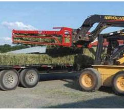
Loader-mounted "Accumagrapple" gathers up 8 to 10 small square bales in the field. Once the bales are gathered together, they can be loaded onto a truck or trailer, with the same piece of equipment.
