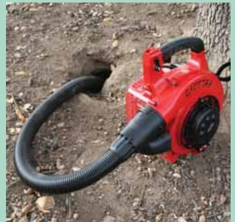
**Gas-powered Cheetah uses a small engine and fan to push exhaust fumes into pest tunnels.**
