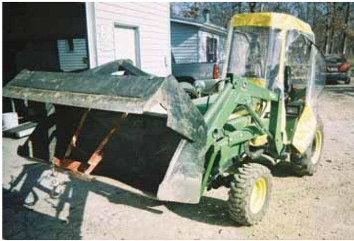
LaVier Schliefert added a hinged top to the loader bucket on his Deere 855 utility tractor. A welded-on grader blade forms the top's cutting edge.
