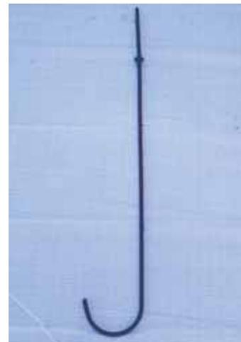
Plastic is held in place with 3-ft. long J-rods spaced 3 to 4 ft. apart around the silo wall.
