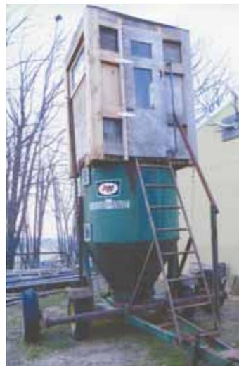
Don Keen converted an old Artsway feed grinder into a portable deer stand by building an enclosure that mounts on top of it 10 ft. off the ground.
