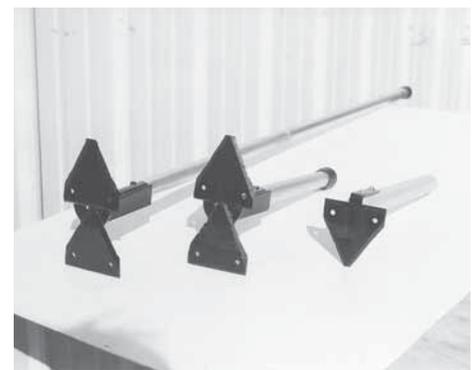
Terry Morgel makes garden hoes from used sickle sections. Two hoes have double sickle sections welded to a large flat washer.
