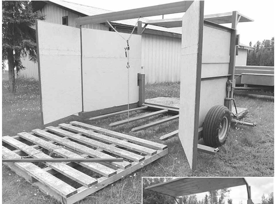
**Pallet slips over 4 long forks to form cart's floor. After bales are loaded, Keddie lowers forks to ground, then drives forward to leave pallet in the field.**
