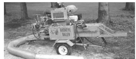
Miller mounted a 38-hp gas engine on the baler to power a 26-gpm pump. It is more than sufficient to power the plunger, knoter assembly and the vacuum with its 14-in. diameter flexible hose. The hose can be used freehand or mounted to a pickup attachment.
