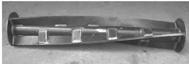
**Rock beater has a spiral shape, which ensures that 70 percent of the opening in the beater is always open so crop can flow smoothly into rotor.**
