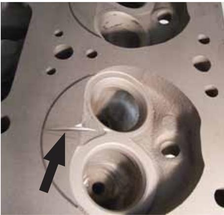
Grooved cylinder heads are said to boost power and result in better fuel efficiency.
