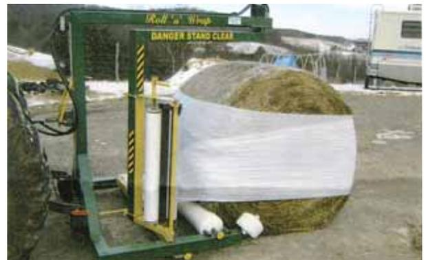
**Instead of a roller table to rotate bale while it's wrapped, operator simply pushes bale along the ground while a rotating arm swings around bale with a roll of plastic.**
