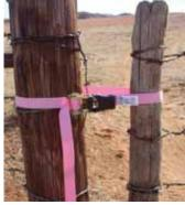
Ratchet strap helps open and close gates secured by tight wire loops. You place strap under wire, then tighten ratchet until wire is loose enough to remove.
