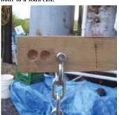
A pair of chains are suspended from an oak board, with each chain supporting a 5-gal. bucket.
