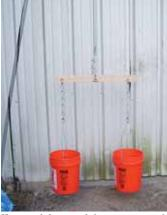
Homemade beam scale is accurate enough to weigh anything from a 50-lb. sack of flour to a soda can.
