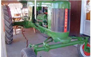
Lloyd Stetson's Oliver 66 "purrs like a kitten" after he repowered it with a 1938 Ford V-8 flathead engine.
