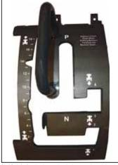
Shift kit includes a lock lever that blocks off the lower 6 gears to shorten up your shift movements.
