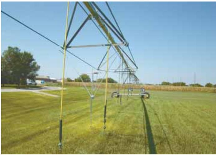
Fenceposts fit onto brackets hanging on hooked rods from center pivot frame.
