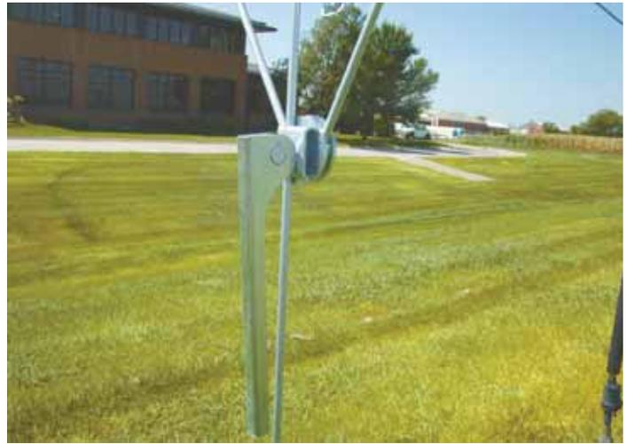
Height of fence line can be quickly adjusted by raising and lowering posts using hand-tightened clamps.
