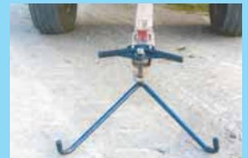
To hook up the wagon, the tractor driver lines the tail rod up anywhere inside the V-shaped rods and backs up. The V-shaped rods slide up and over tail rod.
