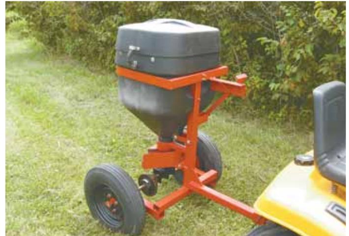
**LeRoy Momper built this 2-wheeled, garden-sized fertilizer spreader using the plastic hopper off a pickup-mounted salt spreader.**
