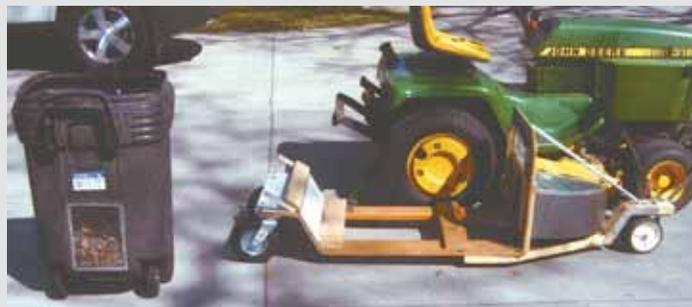
**Cagle's 3-wheeled trailer attaches to discharge side of riding mower, where a 40-gal. plastic garbage can laid on its side (below) collects grass and shredded tree leaves.**
