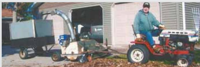
**Marvin Hechel converted an old walk-behind snowblower into this pull-type lawn sweeper. It blows leaves and grass into a homemade trailer.**
