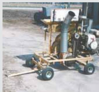
**White sign with red lettering on top serves as a "back-stop" when shoveling leaves into opening on top of machine. Other sign serves as a shield over belts and pulleys.**
