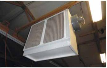
To pull dust from his shop/garage, Noah Hubbard cut out the back side of a surplus wall cabinet, installed 2 furnace filters, and added a small squirrel cage fan.
