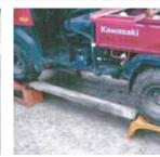
Delbert Hayes made this simple service ramp for his Kawasaki Mule utility vehicle out of 2 sets of car ramps, with planks bolted on between them.
