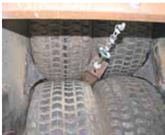
**Nuts drop down through 2 sets of lawn mower tires that run at different speeds to "rub" hulls off (left). Nuts are then fed into a home-built sorting machine.**
