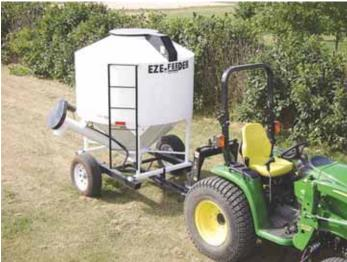
Eze-Feeder grain feeder is available in several different designs for use on everything from pickups to small tractors and ATV's.
