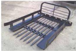
Rock fork has pockets at the rear that ordinary pallet forks slip into. Skid loader's tilt control creates a pitching action that sends rocks to back of unit.
