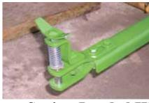
Compression spring holds hitch pin down so it can't shake or rattle.
