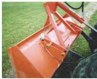
Triangle-shaped steel bracket is welded to back side of loader bucket for 3-pt. hookup. A hydraulic cylinder is used to tilt bucket up or down.
