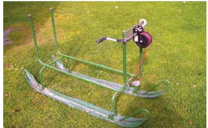
Don Bogardus uses an electric winch to tow this home-built firewood sled up to his house. Hand-cranked winch on sled serves as a backup.
