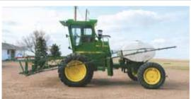
**Daryl Dirks built** this self-propelled sprayer out of an old Deere 7700 combine for \$12,000 and a lot of time. It's equipped with a 60-ft. boom and 750-gal. tank.
