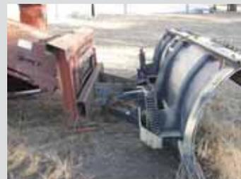
He welded an old county snowplow to the mounting brackets from a grain platform so he can use the combine to plow snow.
