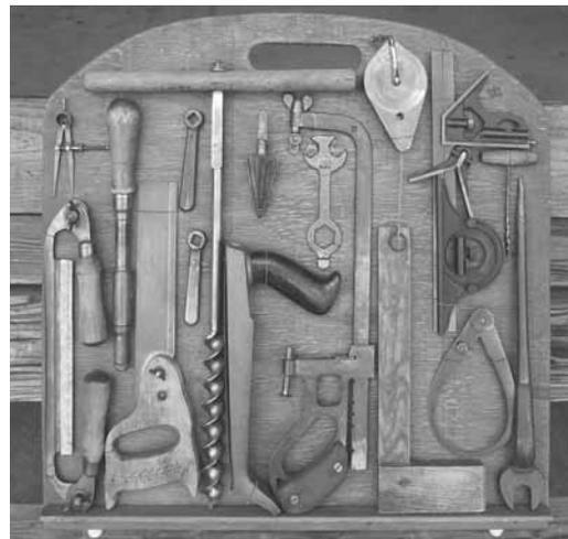
Narrow shelves secured with brass screws support the tools, along with thin wire slipped over tools through holes in plywood and twisted tight on back.
