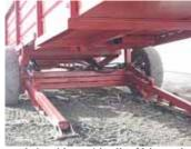
Side view of Olson loading chute (left). A scissors hoist with two 4-in. dia., 30-in. stroke cylinders raises chute up to 11 1/2 ft.
