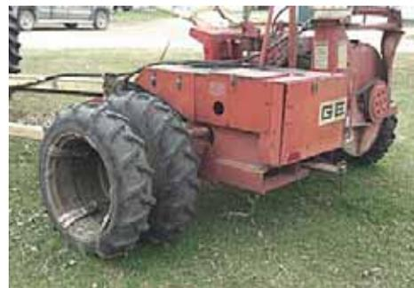
Alan Burda dualed the left wheel on his Gehl 800 2-row silage chopper, adding a 15-in. spacer. “It helps the machine track through muddy corn ground,” he says.
