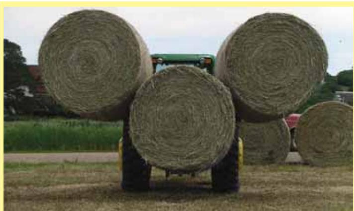
Schreurs 3-bale handler has wings on both sides so bales can be lifted off ground before spearing the middle bale.
