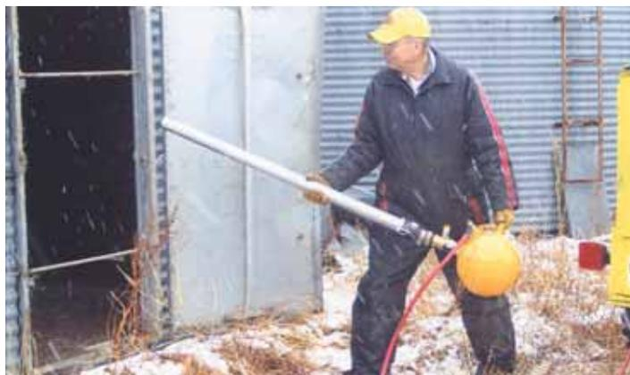
Life Saver uses a blast of compressed air and a 4-ft. long steel exhaust pipe to propel ice cube “bullets”, which dislodge grain from outside the bin.
