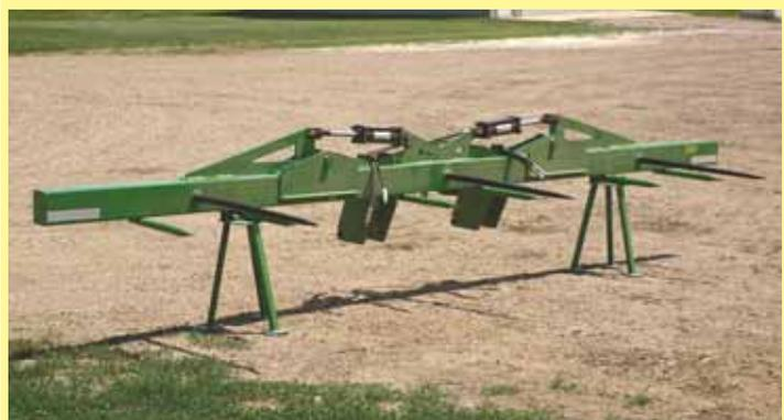
Two long spears go through each bale for stability. Wings fold up when traveling on the road or through gates.
